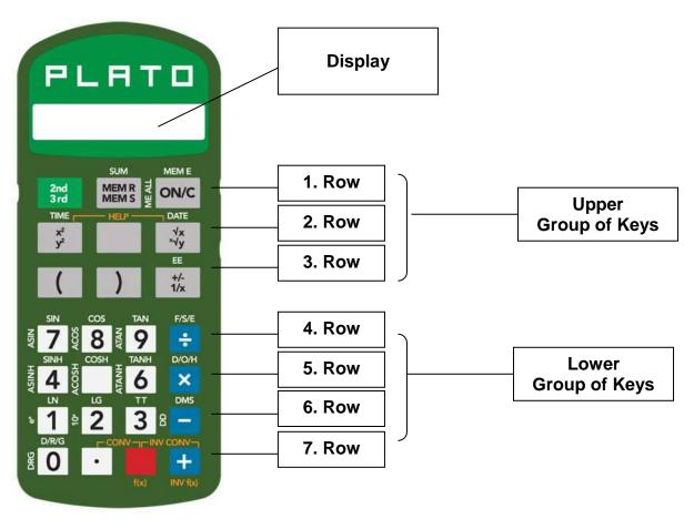
The button in row 1 column 1 has a shift function as known from a PC. A short press activates the second level (layer) of functions connected to the buttons and pressing long activates the third level.
