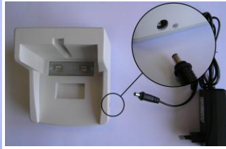
Connecting power supply to the docking station
