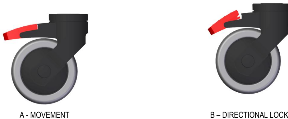
Figure 5 - Directional lock of the castors in the frame
